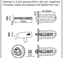
Installation sample for concrete ceilings/walls:
